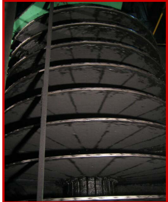
View of the running filter. The Boozer replaces 3 old drum filters and has a solids capacity of 320 kg/m 2 h ( x_{50} < 60 \mu\text{m} , C_{\text{solids,feed}} = 278 \text{ g/l} )
