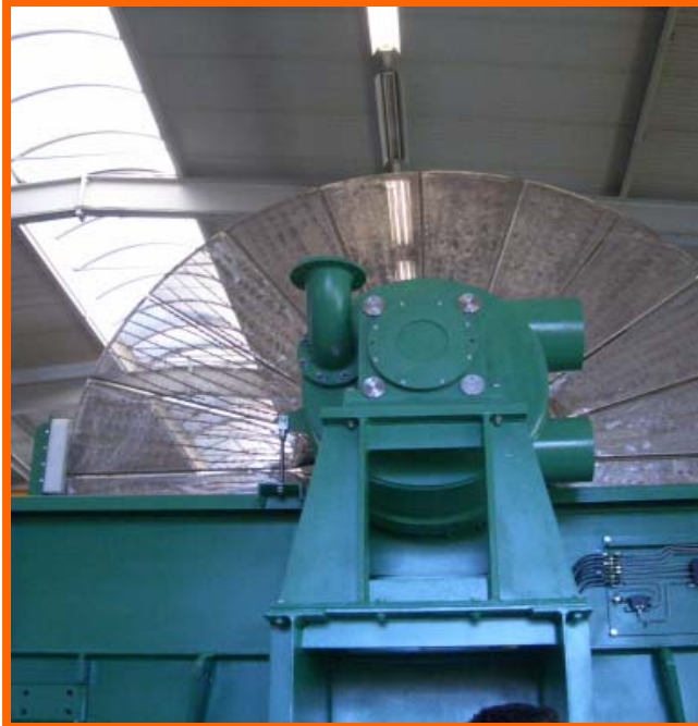
Trough of Boozer ME-Type ( 8 discs, 140 m 2 filter area) in the workshop
