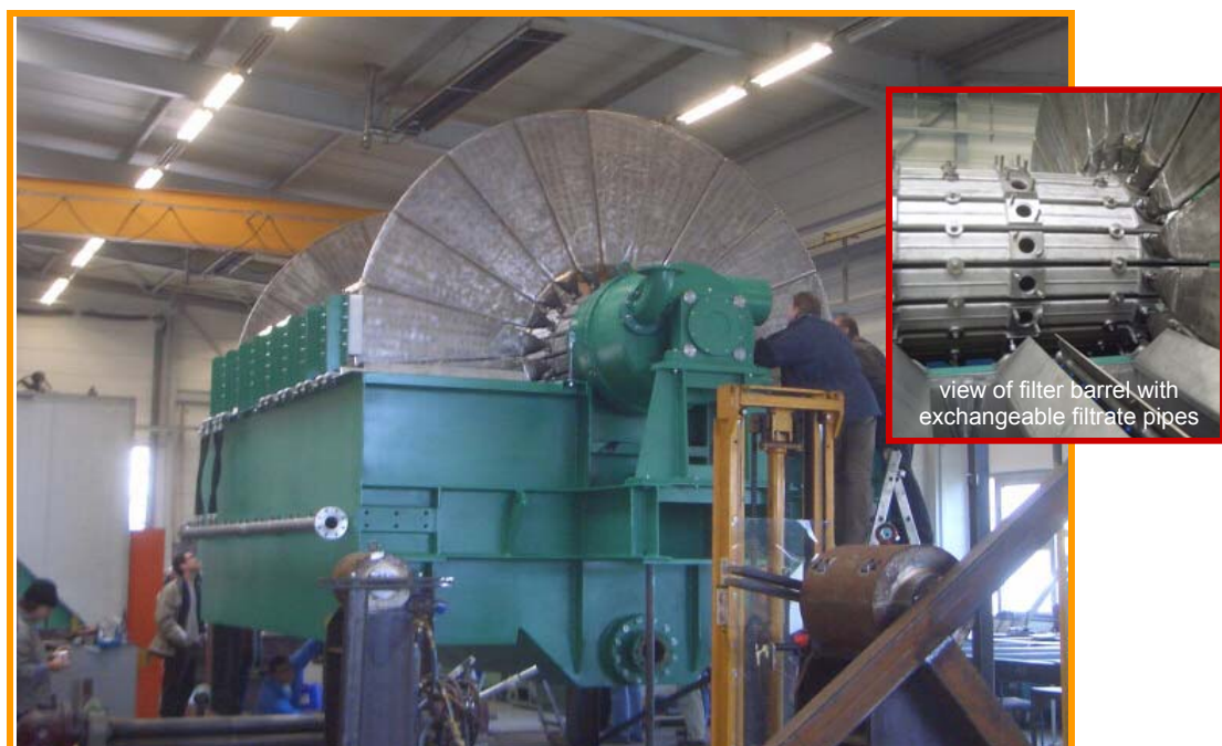
Boozer ME-Type for coal filtration with exchangeable filtrate pipes, 8 discs and 140 \text{ m}^2 filter area in the workshop
