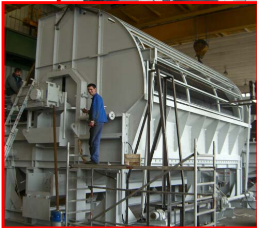
One of two BOKELA drum filters XXL -Type in the workshop ...
