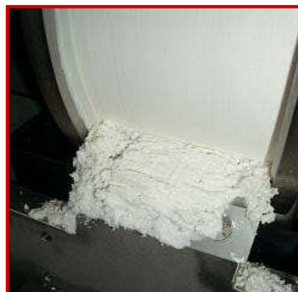
In operation Filter speed: 8 – 24 rpm Manual knife feed: 10 μm steps
