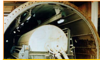
Standard design (large units) with horizontal pressure vessel for bulk materials
