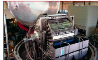
OYSTER-Design (smaller units) with vertical pressure vessel for sophisticated applications (chemical, pharmaceutical and food industry)
