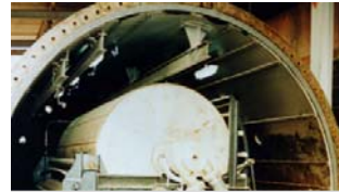
Standard design (large units) with horizontal pressure vessel for bulk materials with high throughput rates
