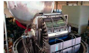
Oyster design (small units) with vertical pressure vessel for sophisticated separation tasks in the chemical, pharmaceutical & food industry, etc.
