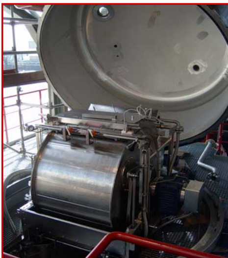
Hi-Bar Oyster Filter with Steam Cabin Filter Area: 3.75 m 2
