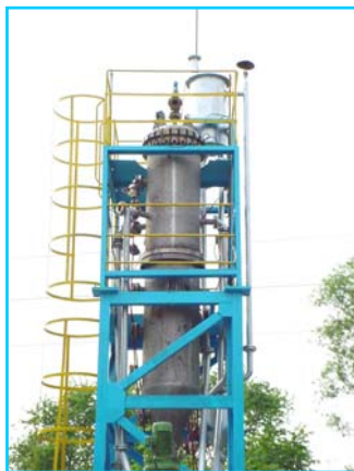
Transportable pilot leaf filter plant (figure left); advanced control and measure systems of the pilot leaf filter (figure above)
